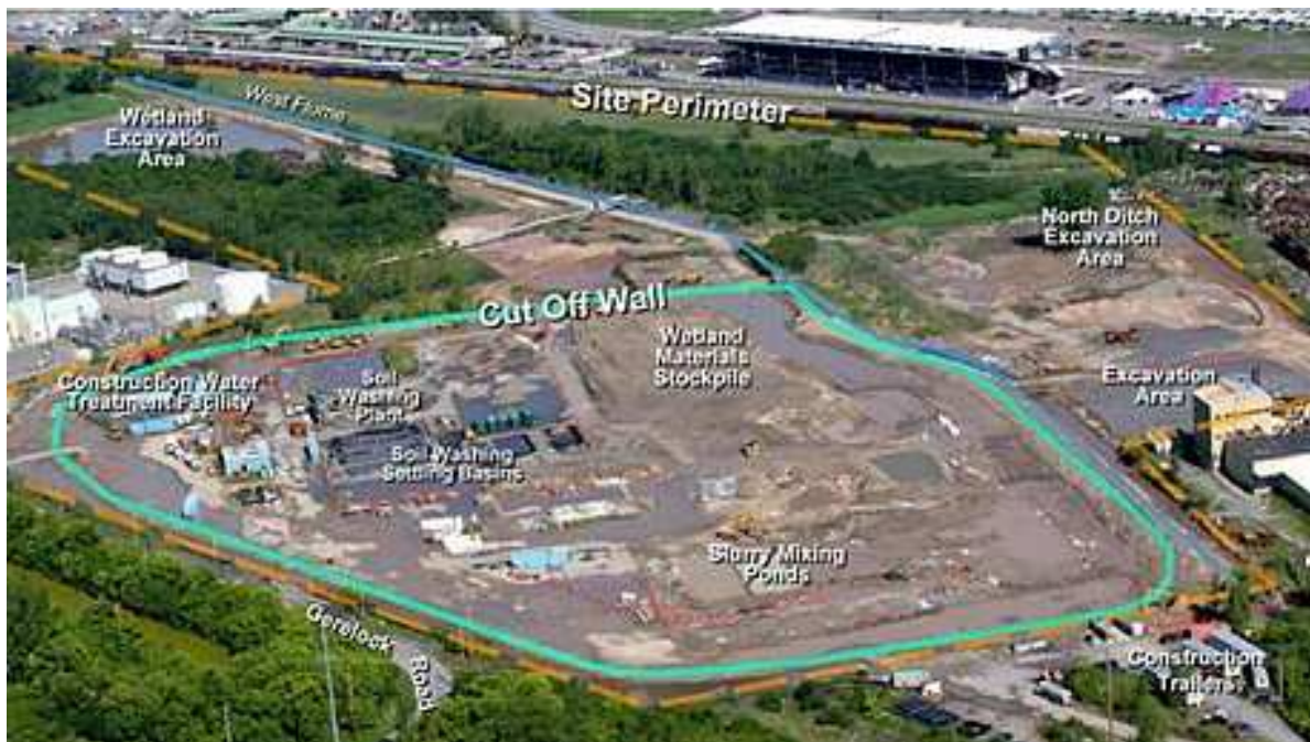
Figure 2. An aerial photo of the LCP site when surface soils were being processed to remove mercury. The Grandstand at the NYS Fairgrounds can be seen in the background. The turquoise line shows the approximate placement of the slurry wall which is designed to prevent contaminants from leaking off-site. The wall consists of a trench dug ~50 ft into the earth, filled with bentonite clay.
